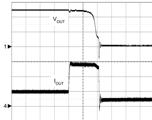
Over Current Protection
